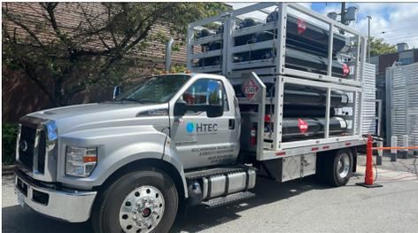
Modular gaseous hydrogen storage system for distribution, ground storage, or as part of a mobile fueling system when integrated with HTEC's PowerFill Gas Transfer Module.
