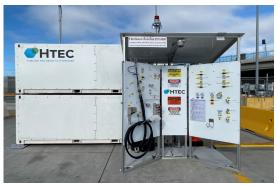
A mechanical hydrogen dispenser capable of fueling H2 vehicles of various storage sizes including yard and drayage trucks, buses, and longhaul tractors, as well as providing backup fueling for light-duty vehicles.
