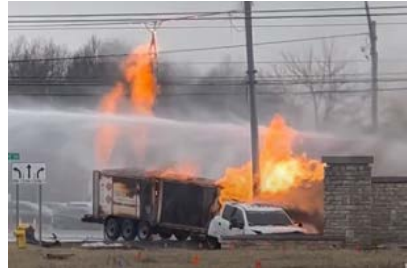
Gaseous hydrogen tube trailer with TPRDs activated. Water mist over trailer keeping tanks cool.
